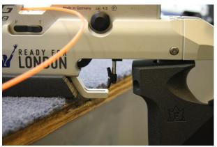
**Trigger extension:** trigger is inside the dimensions of ISSF Rule 7.4.4.1 and protected by a trigger guard.
