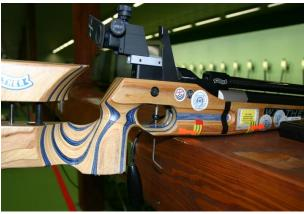
**Trigger adaptation:** trigger is outside the trigger guard and outside the dimensions of ISSF rule 7.4.4.1
