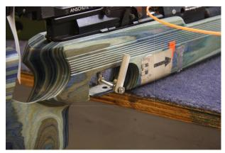
**Trigger adaptation:** trigger is outside the trigger guard and outside the dimensions of ISSF rule 7.4.4.1
